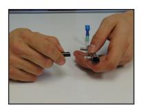
Insert a piece of clear tubing at one end of the cell and place the open end in a cup of warm water. At the other end of the cell, insert a piece of eight-inch clear tubing fitted with the plastic syringe. Now we're ready to flush the cell.
