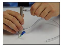
Pull back the syringe to draw water into the cell and push in to flush water back out. You'll need to continue this process until the water in the cup is completely clear.
